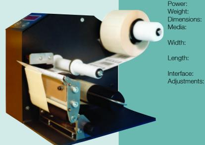
AC Adaptor 230V AC - 24 VDC/500mA. Stepper Motor 5.6kg 260 mm (L), 210 mm (W), 230mm (H) Label roll with 40mm and 76 mm core. Outer diameter 200mm Minimum width: 20mm, Maximum width: 130mm. Minimum length: 25mm, Maximum length: 220mm. Digital for automatic connection Sensor for I Mark and GAP labels. Offset of +30mm/-5mm Switch for GAP or I Mark Power Switch Height adjustable Dispense Bar
